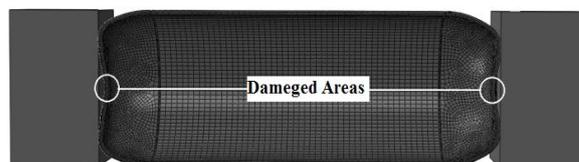
Fig. 3: Deformed model of the cylinder after vertical collision.
