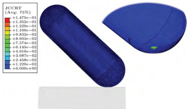
Figure 18. The deformed cylinder model and critical area after oblique drop test.
