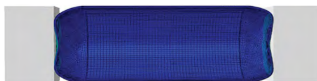
Figure 4. Deformed model of the cylinder after front collision.
