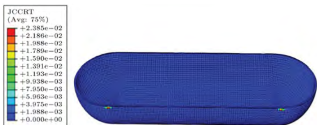
Figure 17. Critical area after side drop test.
